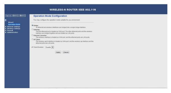
6. after confirm the mode is Bridge, please disconnect the wireless connection.
